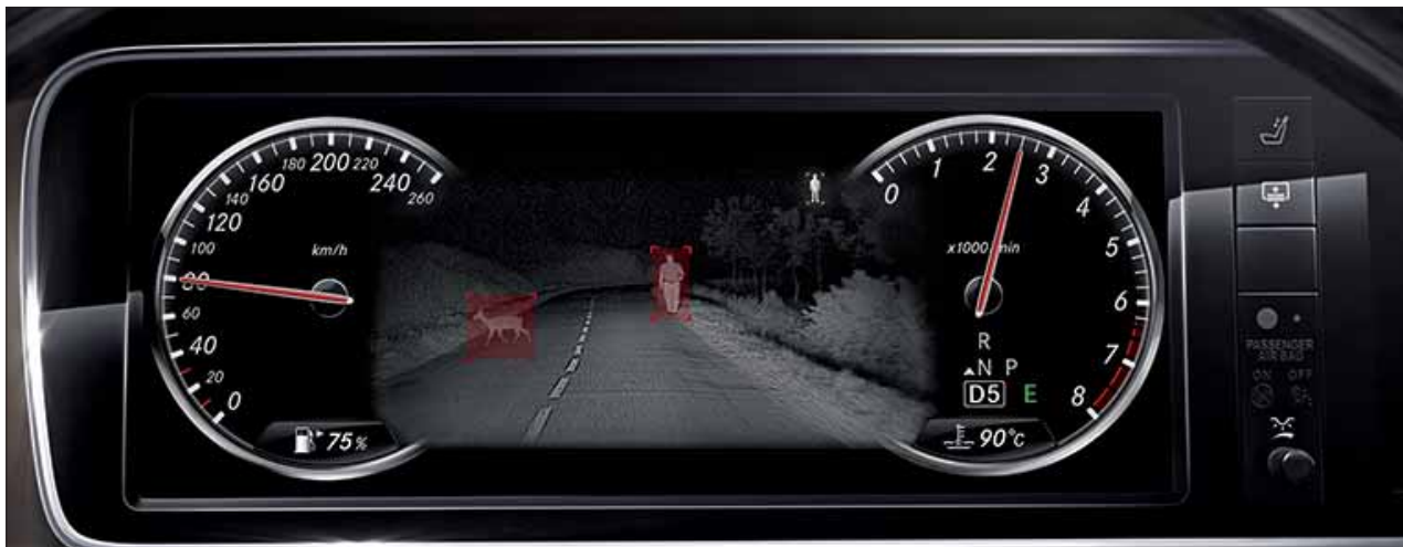
Night View Assist Plus highlights any people it has recognised and helps the drivers to react quicker to dangers by night.
