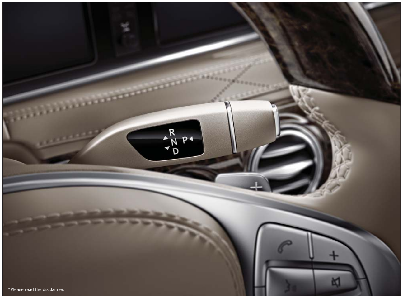
DIRECT SELECT lever on steering column. The driver can also change up or down a gear manually using the additional shift paddle.
