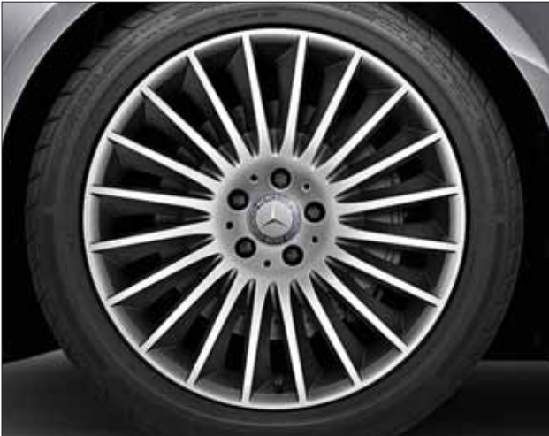
Multi-spoke alloy wheel with 245/45 R 19 front tyre and 275/40 R 19 tyre for the rear for S 500
